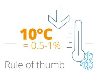
For every 10°C decrease in charge air temperature, SFOC goes down by approximately 1.5 g/kWh. Decreasing charge air temperature through these defouling initiatives could save up to 0.5-1% in fuel consumption, translating into considerable cost savings.
