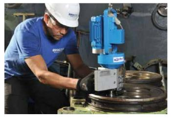
**Workshop refurbishment of engine parts**Refurbishment of valves and valve seats, cylinder heads, cylinder liners, injectors, charge air coolers, etc.
