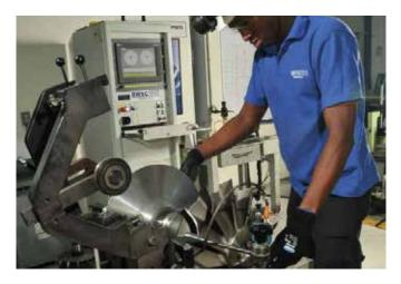
**Turbocharger service and maintenance** Turbocharger service, cleaning/sandblasting, re-blading, balancing of rotors, etc.
