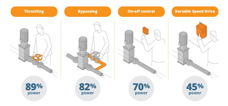
**Variable Speed Drives** (VSDs) ensure the pump is delivering only the necessary flow. Installing VSDs on pumps and fans helps avoid unnecessary energy consumption.
