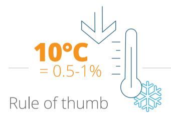
For every 10°C decrease in charge air temperature, SFOC goes down by approximately 1.5 g/kWh. Decreasing charge air temperature through these defouling initiatives could save up to 0.5-1% in fuel consumption, translating into considerable cost savings.
